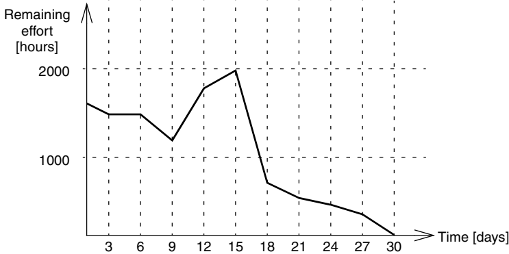
Figure 14-15 Assessing progress trend with a burn down chart. An increase corresponds to an upward revision of estimated work (new work, tasks initially underestimated). A decrease corresponds to a downward estimate of remaining work (work completed, obsolete tasks taken out of the plan).
