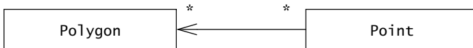
Figure 2-24 Example of a one-directional association. Developers usually omit navigation during analysis and add navigation information during object design, when they make such decisions (see Chapter 8, Object Design: Reusing Pattern Solutions , and Chapter 9, Object Design: Specifying Interfaces ).
