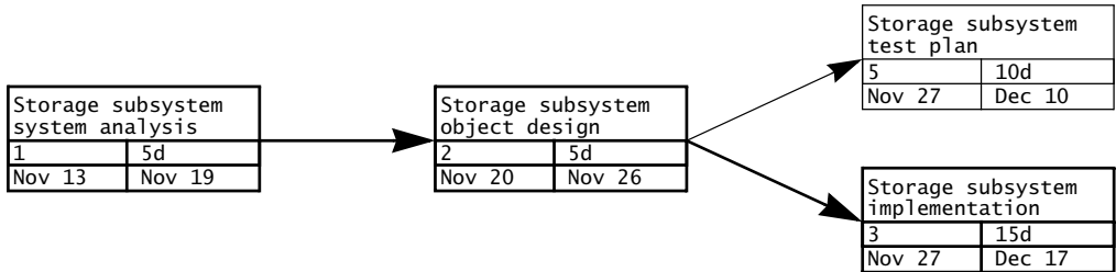
Figure 3-11 Schedule for the database subsystem (PERT chart). Thick lines denote the critical path.
